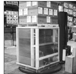
The new packaging system provided exceptional stackability when a 900-lb. load was placed on top of it.
