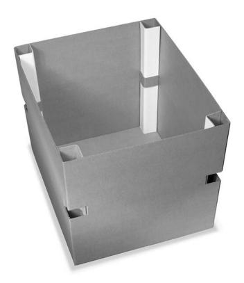
Making two parallel die-cuts in each corner of a corrugated carton and pushing the resulting band inward is an easy, economical way to hold VBoard® edge protectors in place without the use of additional materials such as strapping or glue. Positioning the VBoard with its outside edge toward the inside of the carton, as shown, provides other advantages too.
