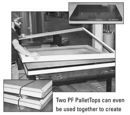
trays and lids for heavy, thin, rectangular products like the industrial floor scale above. A sheet of particleboard is placed in an upside-down PF PalletTop to create the bottom tray into which the product is loaded. Another sheet of particleboard and second PF PalletTop go on the top, and the entire load is strapped at the edges.
