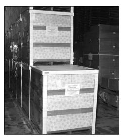
PF PalletTops can be used on the top of a load to hold VBoard® in place during stretch-wrapping. It's a great combination that helps stabilize and unitize the load during shipping and handling. The strong framework created by the PF PalletTop and VBoard also provides stackability for pallets of lightweight products.
