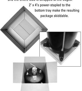
A PF PalletTop used in the bottom of a box prevents sharp objects, like the feet of this drain caddy, from poking through the corrugated.
